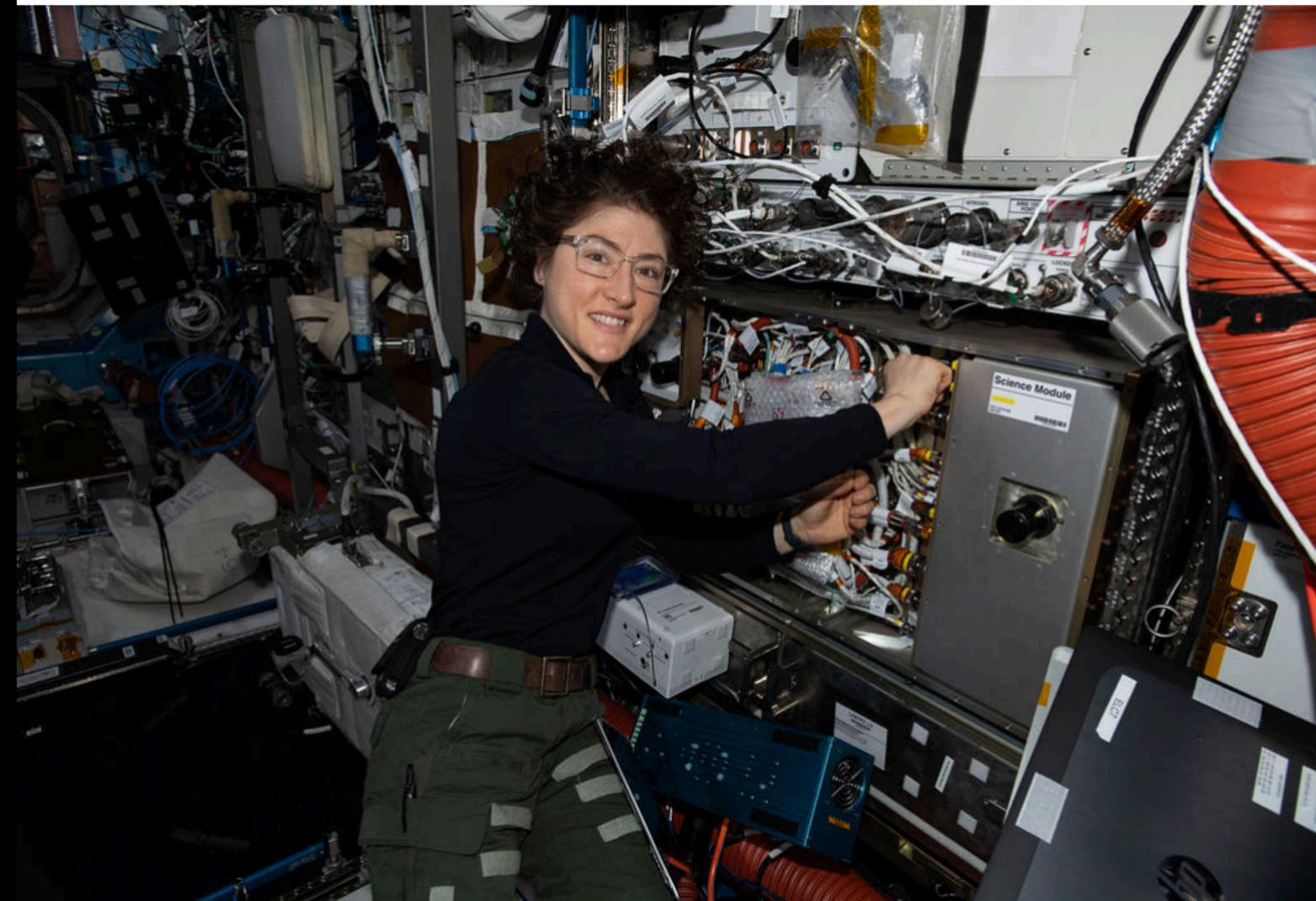
iss061e145487 (Jan. 28, 2020) --- NASA astronaut and Expedition 61 Flight Engineer Christina Koch works on the Cold Atom Lab (CAL) swapping and cleaning hardware inside the quantum research device. The CAL enables research into the quantum effects of gases chilled to nearly absolute zero, which is colder than the average temperature of the universe.
